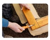
(11) Lay out pieces of cardboard from your packaging to protect your trim. Arrange the four trim pieces so that each arrow points outward. Apply water resistant wood glue to the dowels, and insert into the short trim pieces. Apply a thin coat to **both surfaces** of the corner joint including the dowels. Use a 1%" screw to draw the joint tight.
