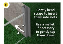
Now, install the included metal straps between each joiner bracket. Gently bend the straps, as needed, to insert them into the slots. This will keep the sides of your raised bed from spreading during installation and later when you fill it with soil.
